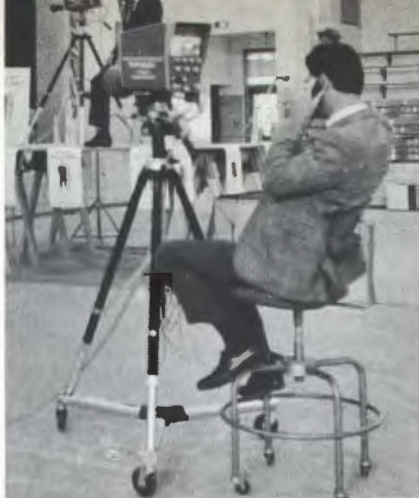
Two small viewfinder cameras in use here offer flexibility, but don't expect them to compete with the big cameras and heavy dollies in the studio or on remotes.
