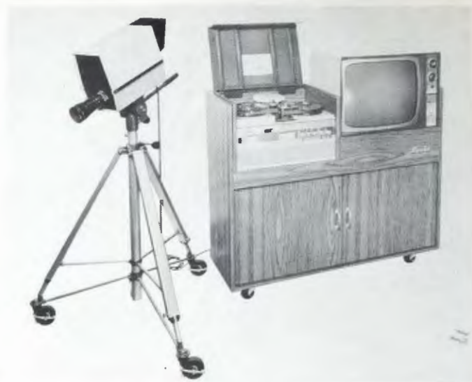
Fig. 3 This basic system includes a camera, videotape recorder, and monitor. Many major manufacturers are now offering origination packages to fit the needs of the low, medium and large budget system.
