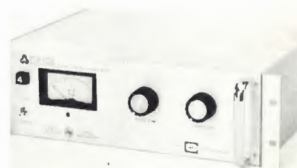
Fig. 4 Example of color TV modulator with audio and video level controls.
