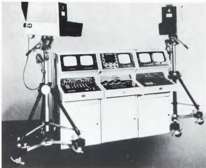
Fig. 2 Packaged system with the console as the key unit. Emphasis is on live originations in the studio.
