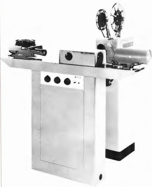
Three-way optical multiplexer.
